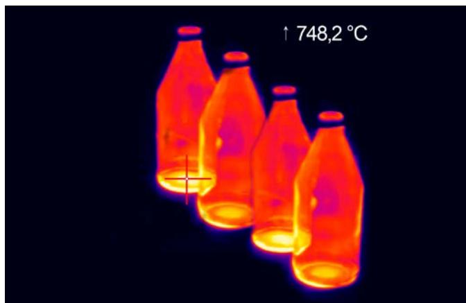
Hot spot detection at glass bottle production
