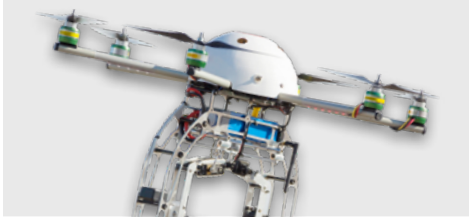
Possible extension with GoPro Hero camera, GPS USB flashdrive and 2.4 GHz flight control receiver
