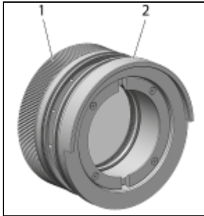
Figure 16: Focusing unit (external and internal part)
