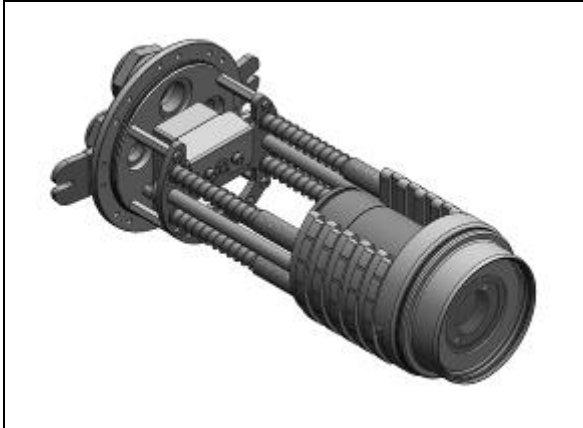
Figure 37: Front part with infrared thermometer
