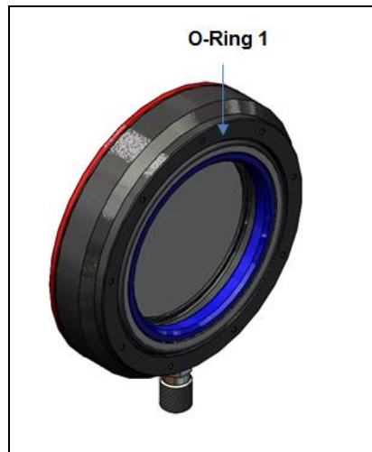
Figure 31: Insert O-ring 1 in air purge collar
