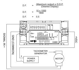
Since the division factor falls between 1.2 and 10.5, DIP switch position S2 is set to the "ON" position, according to the Division Factor Selection Chart. To scale the CUB4 Voltmeter, the motor is run at full speed and a calibrated
