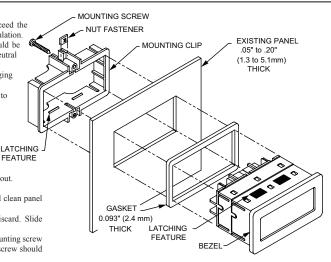
Visually inspect the gasket for proper seal. The gasket should be compressed approximately 75 to 80% of its original thickness. (Recommended torque is 28 to 36 in-oz.)
