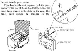
farthest forward slot possible. To achieve a proper seal, tighten the latch screws evenly until the unit is snug in the panel (Torque to approx. 28 to 36 in-oz [0.202 to 0.26 N-m]). Do not over-tighten the screws.
