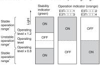
If the E3T fs operating level is set to the stable operation range, the E3T will be in most reliable operation without being influenced by temperature change, voltage fluctuation, dust, or setting change. If the operating level cannot be set to the stable operation range, pay attention to environmental changes while operating the E3T.
