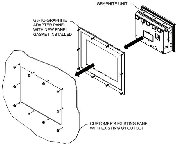
\*The mounting clips may or may not need the mounting foot removed in certain installations, depending on how close the Graphite cutout is to the original G3 cutout.
