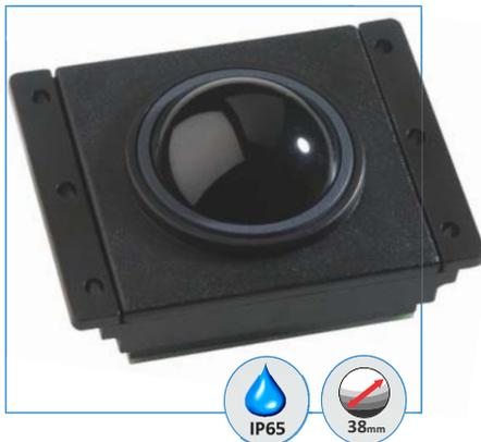
The GK38 series are ruggedised professional trackballs for harsh industrial environments. The double-sided seal ring provides a sealing to IP65 static (ball in rest). Stainless steel shafts and bearings ensure a solid and precise pointer control. The unit can be used for frontpanel mounting (remove the mounting bracket) or for backpanel mounting.
