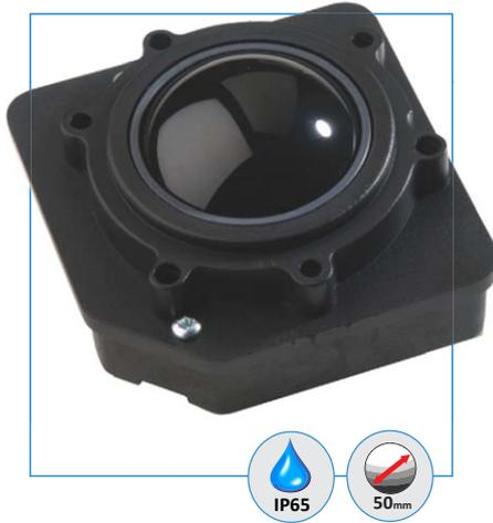
The GK50 is a high specification keyboard or panel mounted trackball. It is constructed from a glass loaded PBT chassis and benefits from its large diameter shafts for smooth running. The GK50 is sealed to IP65 static (ball in rest). Designed to be panel mounted as part of OEM systems, the GK50 is ideal for demanding applications such as medical equipment, process control, air traffic control and ruggedised keyboards.
