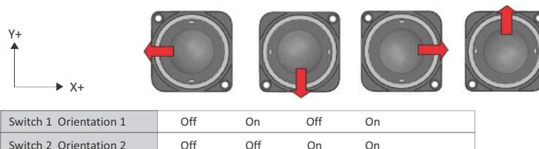
Figure.1 Mounting Orientations
