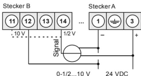
**3-Leiter Sensor 0-1/2...10 V mit 24 VDC Geberversorgung**
