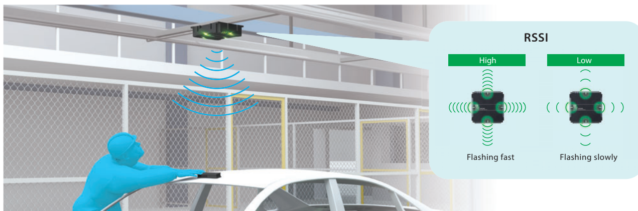
Check the reception level with the indicators on the reader/writer to find the best installation position of an RF tag
